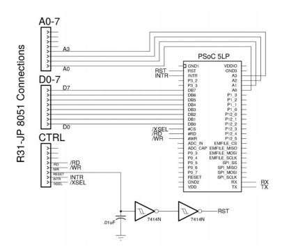
\*Note: Power (5V) and ground (0V) connections were intentionally left off of the PSoC in the schematic for clarity.
