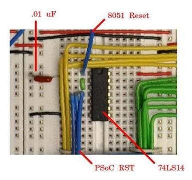
In addition to connecting the RX pin to a UART driving device and the designated pins / bus to the 7 segment display, the three GND pins of the PSoC should connect to the ground of the 8051 system. VDD and VDDIO should be tied to +5VDC.
