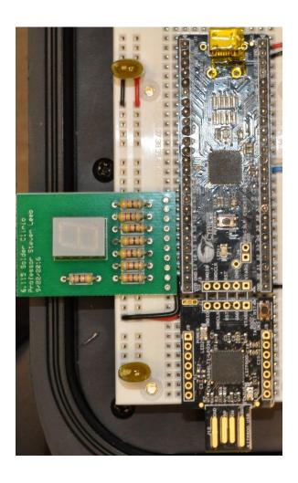
The PSoC Catcher also has a RST line which controls the software reset of the entire PSoC replacement. This RST line should be connected to the 8051 reset pin through two 7414 inverters with a .01 uF capacitance on the 8051 reset line.
