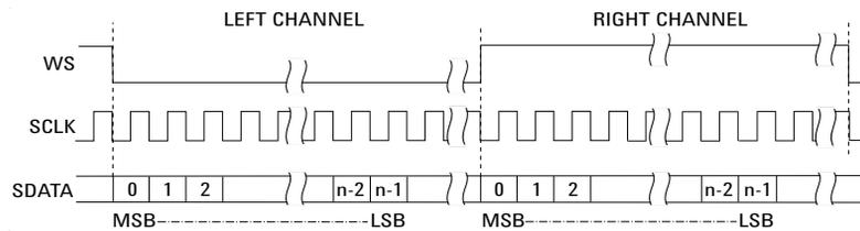
**Right-Justified** – Data transmission (MSB first) is right-justified to the transition of WS.
