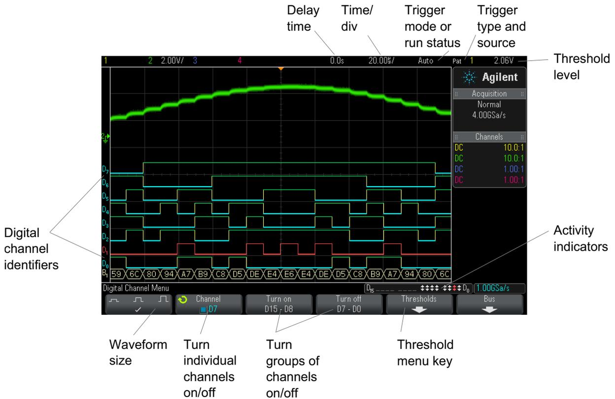
**Activity indicator** When any digital channels are turned on, an activity indicator is displayed in the status line at the bottom of the display. A digital channel can be always high (■), always low (■), or actively toggling logic states (↑). Any channel that is turned off will be grayed out in the activity indicator.
