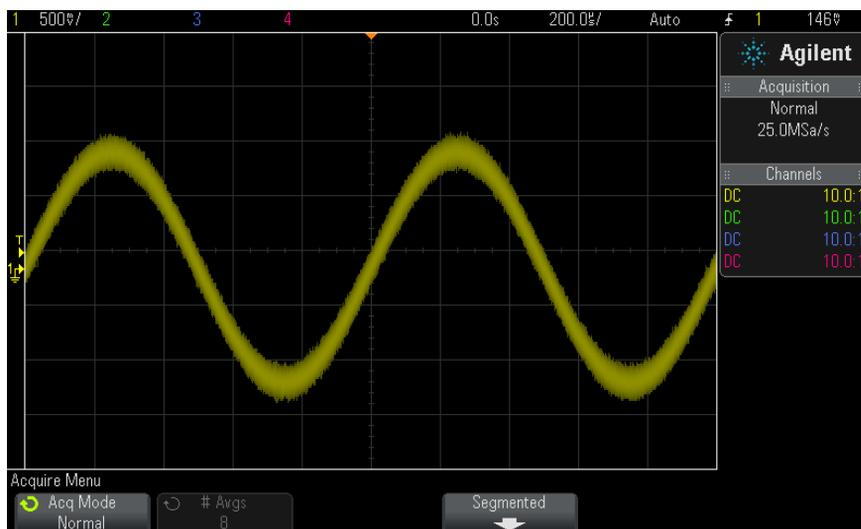
**Figure 38** Random noise on the displayed waveform
