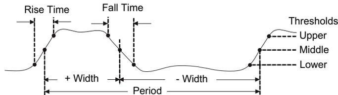
The default lower, middle, and upper measurement thresholds are 10%, 50%, and 90% between Top and Base values. See ["Measurement Thresholds"](#) on page 237 for other percentage threshold and absolute value threshold settings.
