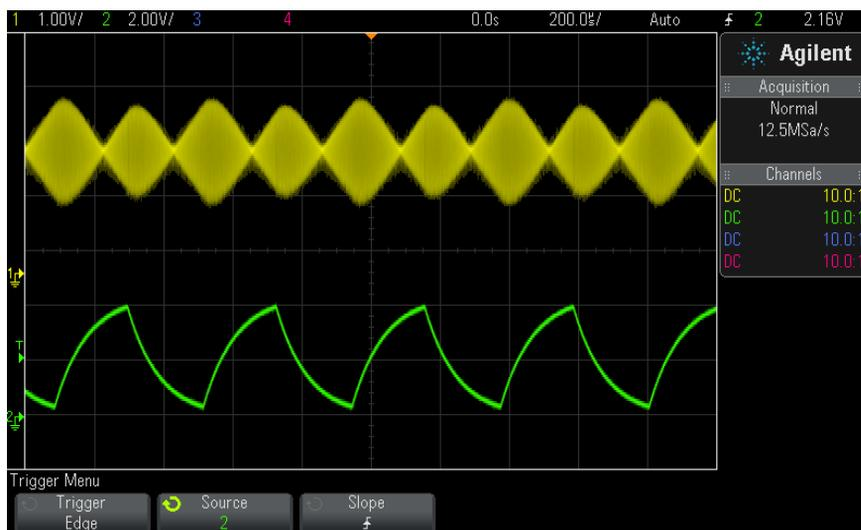
**Figure 26** Amplitude Modulation Shown at 40% Intensity
