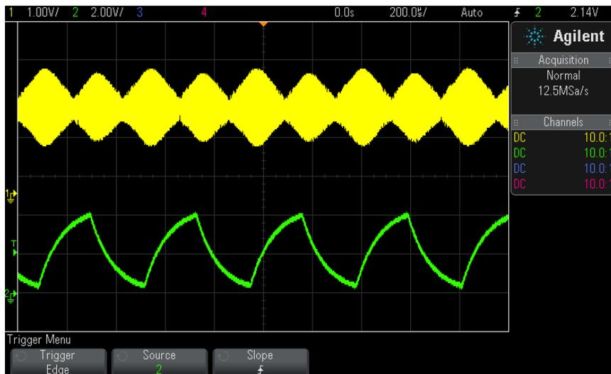
**Figure 25** Amplitude Modulation Shown at 100% Intensity
