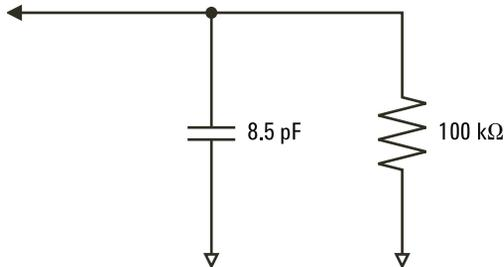
**Figure 21** DC and Low-Frequency Probe Equivalent Circuit
