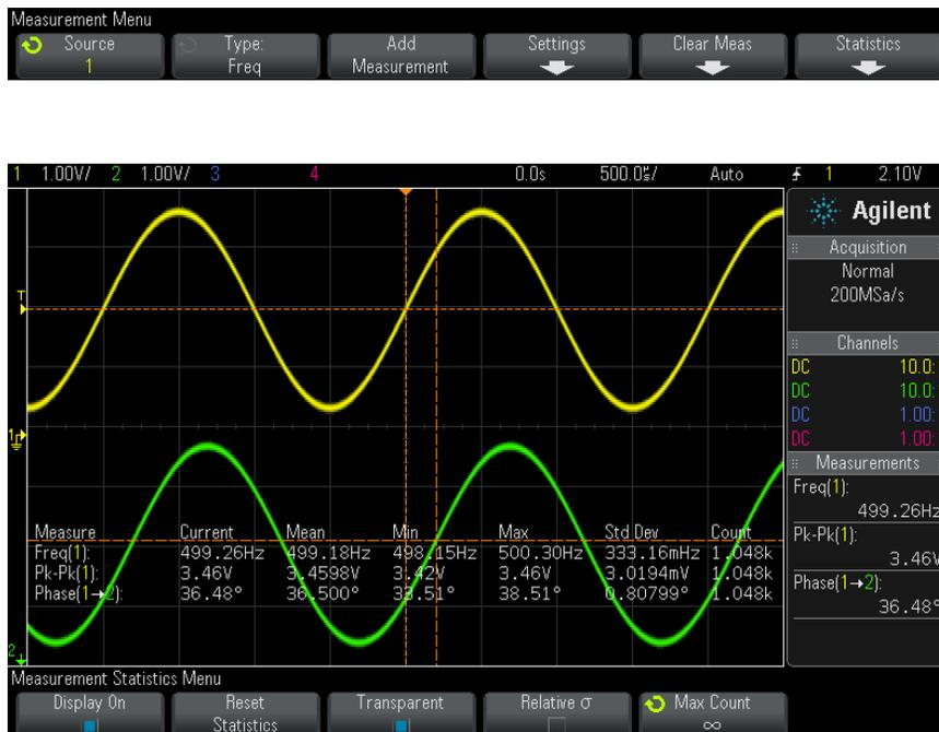
The following statistics are shown: Name of the measurement, current measured value, mean, minimum measured value, maximum measured value, standard deviation, and the number of times the measurement has been made (count). Statistics are based on the total number of captured waveforms (count).
