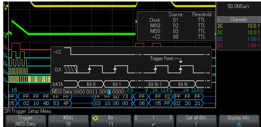
The **Set all Bits** softkey will set all bits in the data string to the value of the **01X** softkey.
