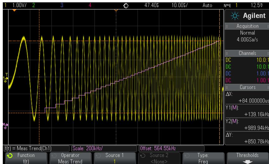
**Figure 17** Example of Measurement Trend
