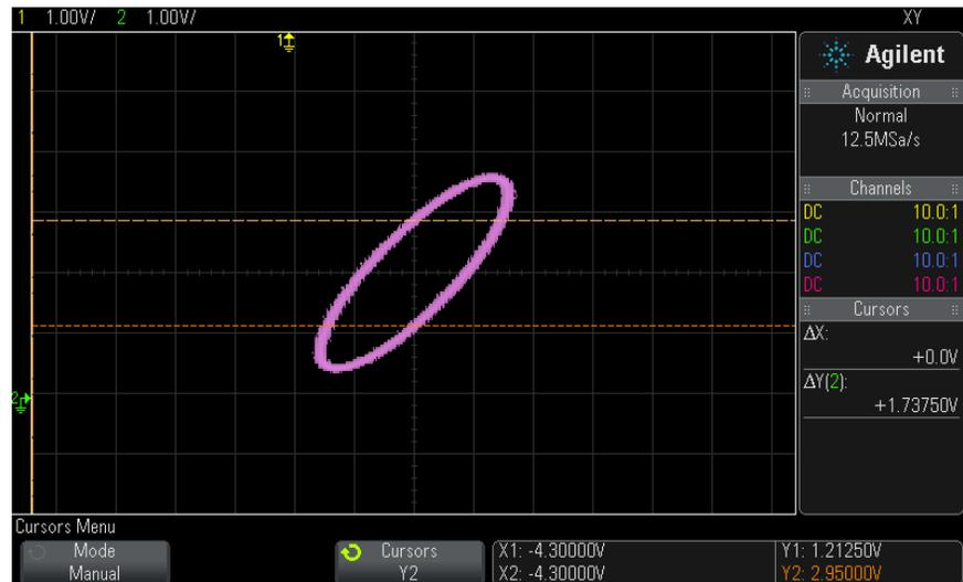
**Figure 4** Phase difference measurements, automatic and using cursors
