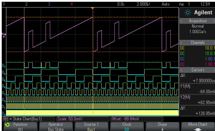
**Figure 19** Example of Chart Logic Bus State
