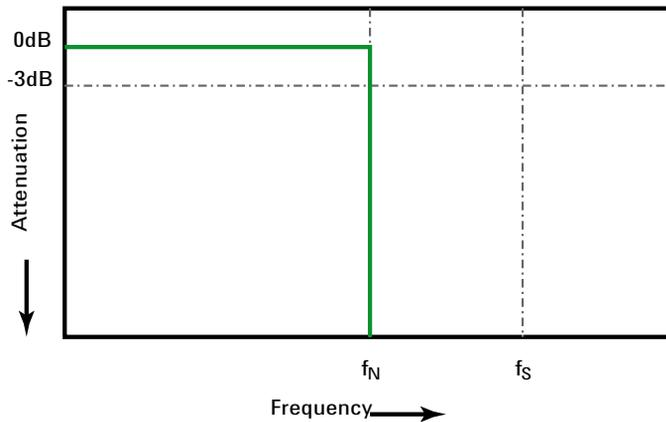
**Figure 34** Theoretical Brick-Wall Frequency Response
