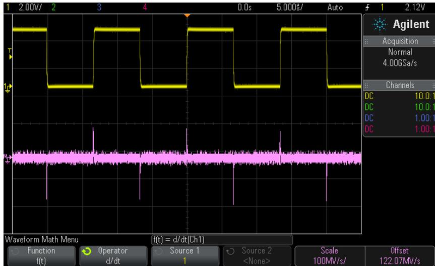
**Figure 7** Example of Differentiate Function
