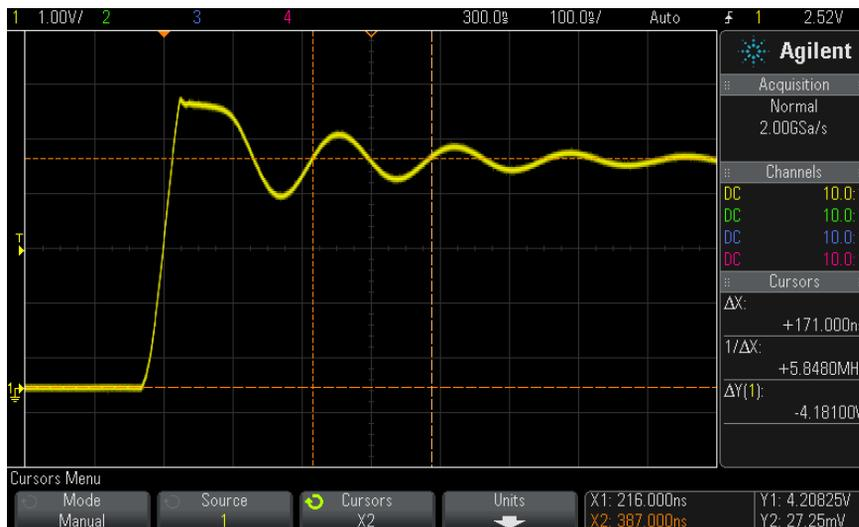
**Figure 41** Cursors measure frequency of pulse ringing
