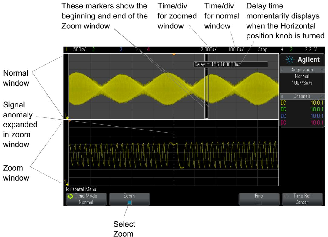
The area of the normal display that is expanded is outlined with a box and the rest of the normal display is ghosted. The box shows the portion of the normal sweep that is expanded in the lower half.
