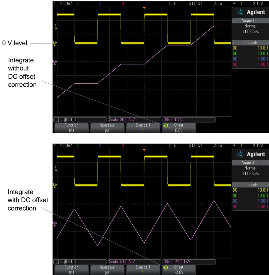
**Figure 8** Integrate and Signal Offset
