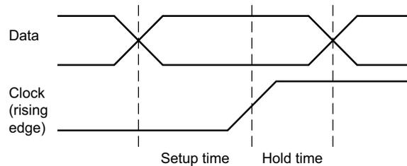
One oscilloscope channel probes the clock signal and another channel probes the data signal.
