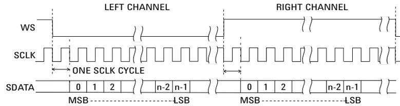
**Left-Justified** – Data transmission (MSB first) begins at the edge of the WS transition (without the one-bit delay that Standard format employs).
