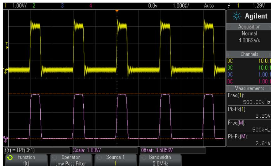
**Figure 15** Example of Low Pass Filter
