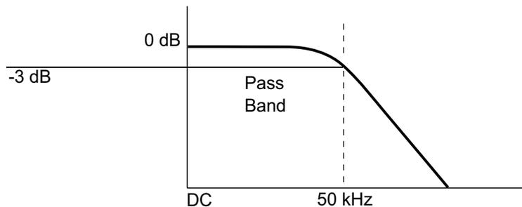
You can use HF Reject to remove high-frequency noise, such as AM or FM broadcast stations or noise from fast system clocks, from the trigger path.
