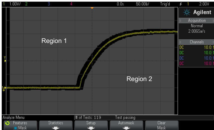
Up to 8 regions can be defined for a mask. They can be numbered 1-8. They can appear in any order in the .msk file. The numbering of the regions must go from top to bottom, left to right.
