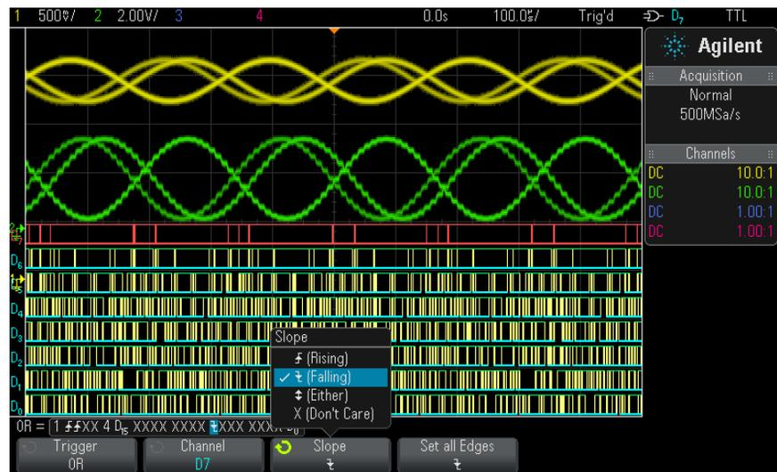
If all channels in the OR trigger are set to don't care, the oscilloscope will not trigger.
