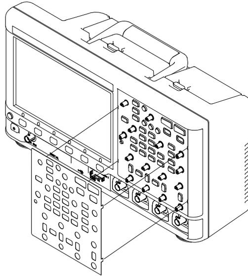
**3** Reinstall the front panel knobs.
