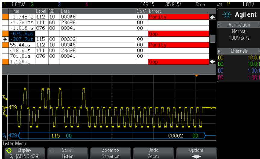
In addition to the standard Time column, the ARINC 429 Lister contains these columns:
