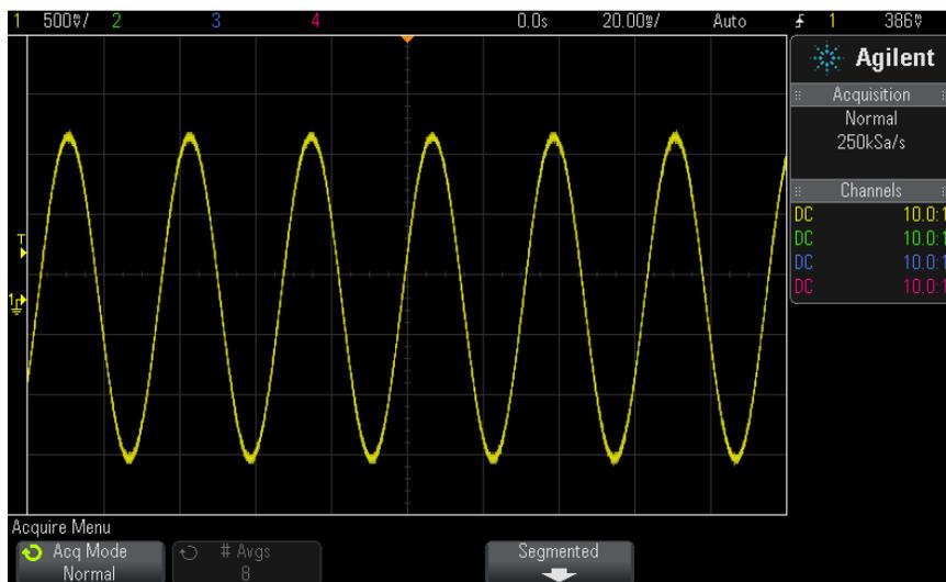
**Figure 36** Sine With Glitch, Normal Mode
