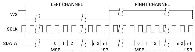
**12** Press the **WS Low** softkey; then, turn the Entry knob to select whether WS Low indicates Left or Right channel data. The on-screen diagram changes with your selection.
