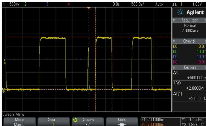
**Figure 43** Measuring pulse width with cursors
