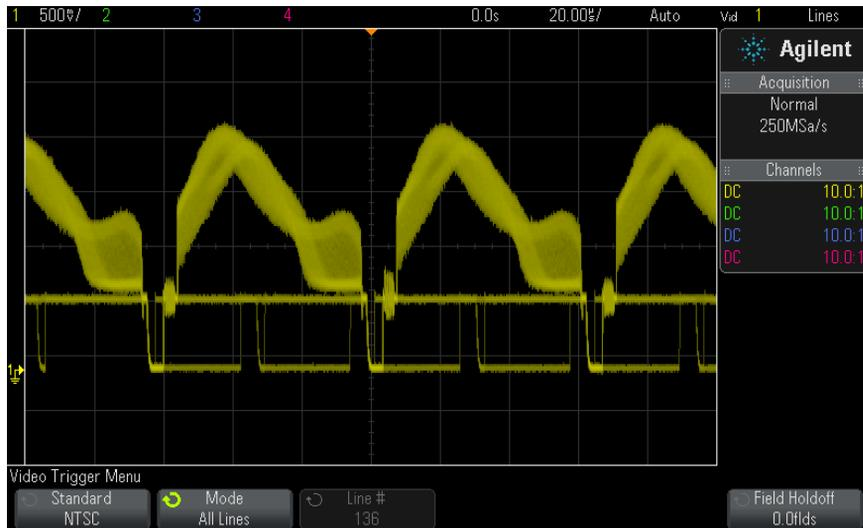
**Figure 28** Triggering on All Lines
