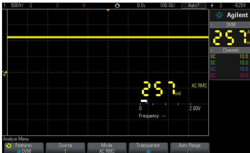
The DVM makes accurate RMS measurements when the signal frequency is between 20 Hz and 100 kHz. When the signal frequency is outside this range, "<BW Limit?" or ">BW Limit?" appears in the DVM display to caution you about inaccurate RMS measurement results.
