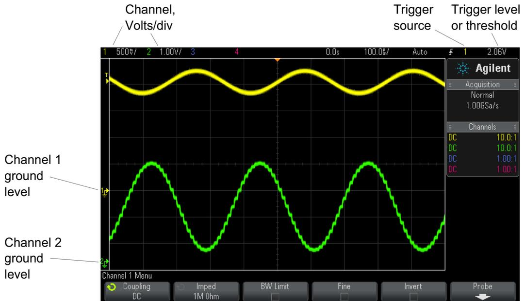
The ground level of the signal for each displayed analog channel is identified by the position of the
