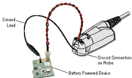
**Figure 45** Measurements on Battery Powered Devices Using the N2820A Probe
