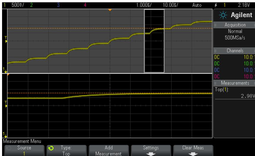
**Figure 46** Isolating area for Top measurement
