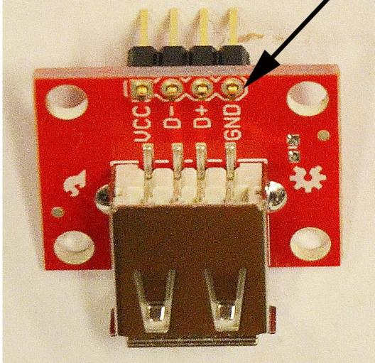
4. Install the connector board, bypass cap, power wiring, and PSoC USB Cable on your kit. Do NOT connect your PSoC evaluation board to anything yet.
