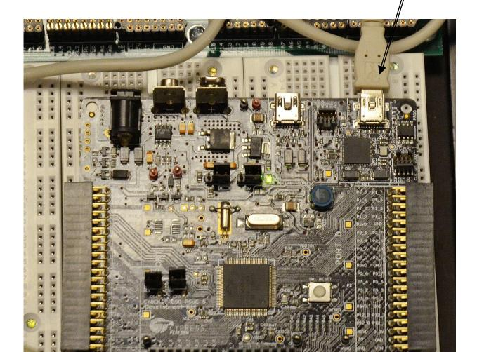
Once your kit has been modified to provide USB power to the PSOC, you can now connect your PSOC to your R31JP using a serial cable and a NULL Modem connector:
