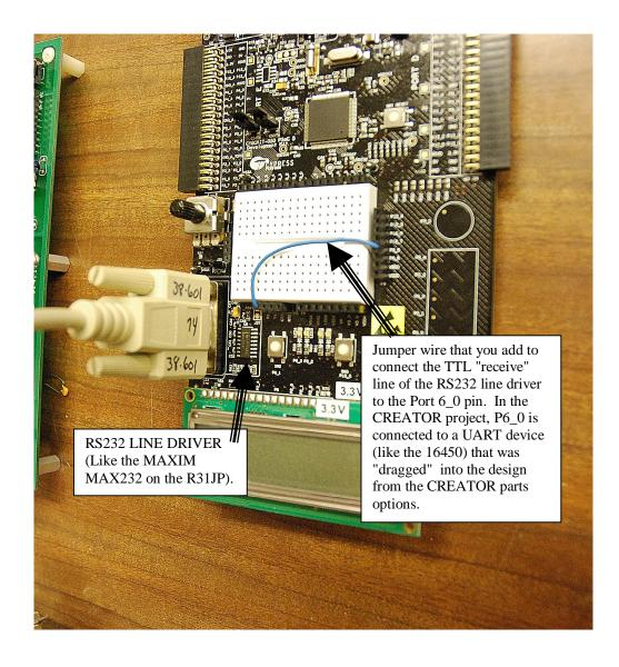
Hereøs a mighty Blackbird with the R31JP sending a serial message to the PSOC. You need to use the NULL modem block as shown in the picture.
