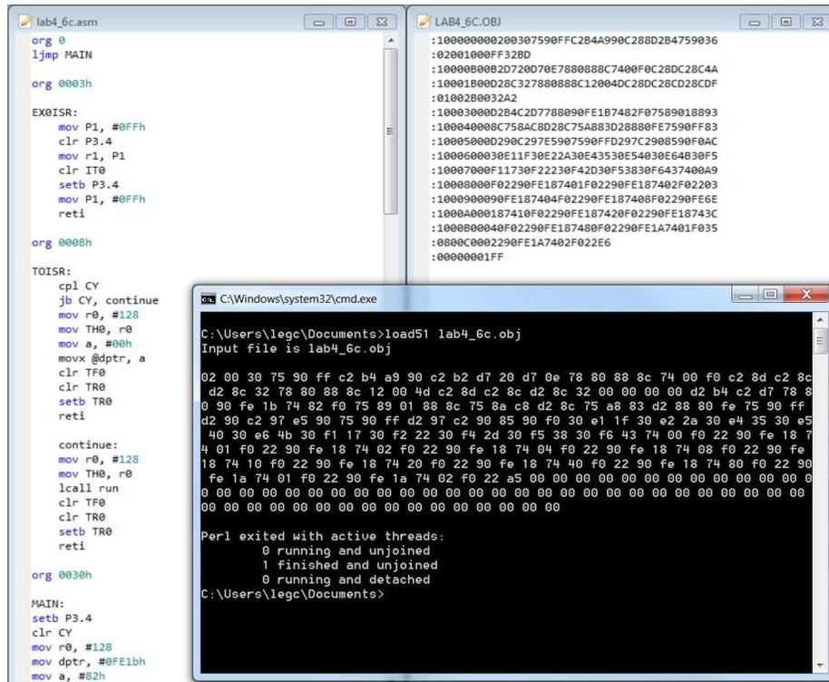
Figure 1 Left: This is an .asm file. Right: The assembled Intel Hex file of the .asm file on the left. Bottom: Loading the code into FreeSoC flash with “load51.”
