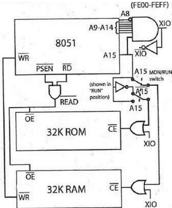
In normal R31JP operation either the external ROM or RAM, accessed by PSEN and RD control signals respectively, can be read from using the combined READ signal (OR for active low signals).
